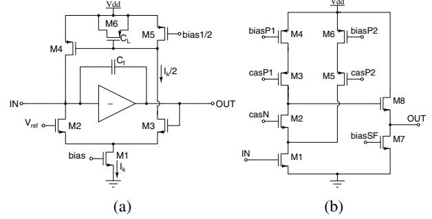
Fig. 3: Transistor level schematics of the CSA feedback circuit (a) and its core amplifier (b).
