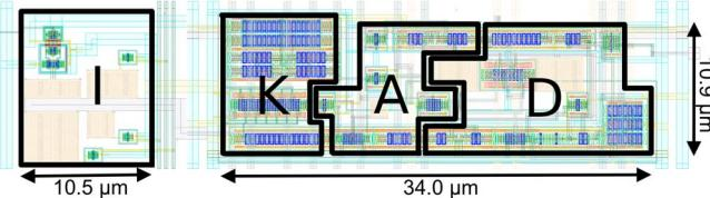
Fig. 2: Layout of a single channel of the proposed front-end. (I) Charge injection, (K) Krummenacher filter, (A) Core Amplifier, (D) Discriminator.
