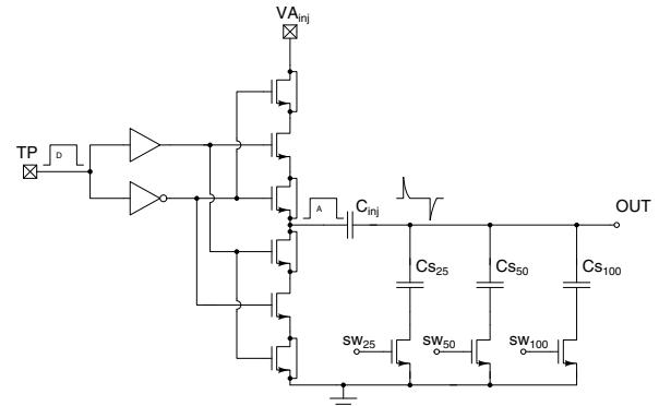
Fig. 5: Transistor level schematic of the charge injection circuit.
