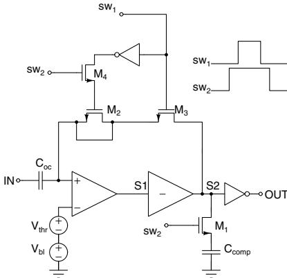
Fig. 4: Schematic block of the proposed LED with offset compensation.
