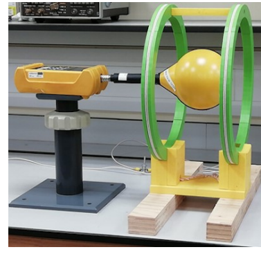
Fig. 10– New calibration facility for magnetic field meters at NPL.
