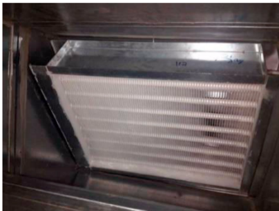
Figure 1. Coated Finned coil for heat and mass transfer
