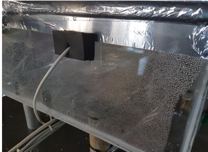
Figure 6. Water droplets formation during condensation are collected in a basin.
