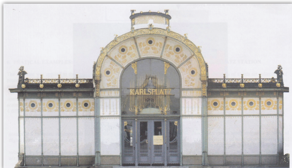
Figure 3. The first architectural true-orthophoto generated by using the "Otto Wagner Pavillon" test material integrated with first point-clouds surveyed by Terrestrial Laser Scanning systems (Boccardo et al, 2001).
