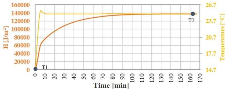
Fig. 3. The heat per unit of the area required by the sample to increase the temperature from T1 to T2;
