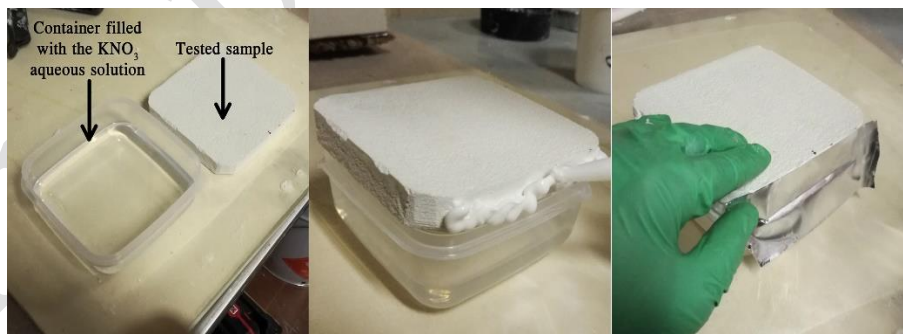
Fig. 4. The cup filled with the saturated solution, the tested specimen and the sealing operation;
