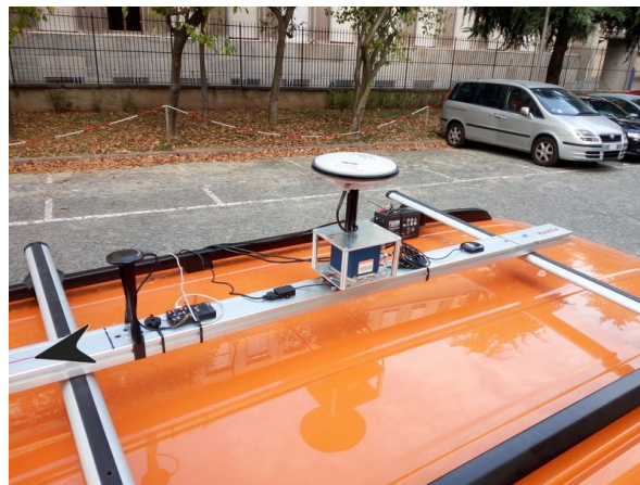
Figure 6. Sensors located on the crosswise bar on top of a vehicle. The black arrow on the left indicates the direction of motion.
