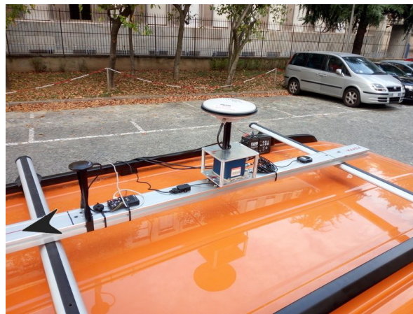
Figure 6. Sensors located on the crosswise bar on top of a vehicle. The black arrow on the left indicates the direction of motion.
