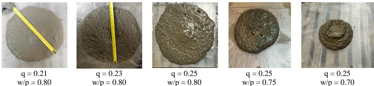
Fig. 3. SC-CBM specimens subjected to flowability tests
