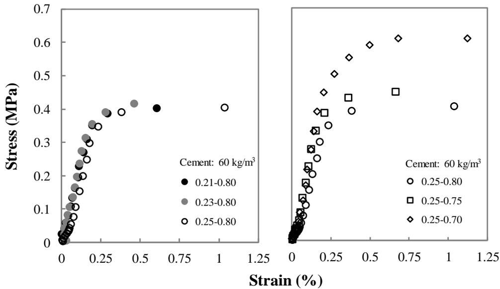
Fig. 6. Stress-strain curves obtained from quick shear tests
