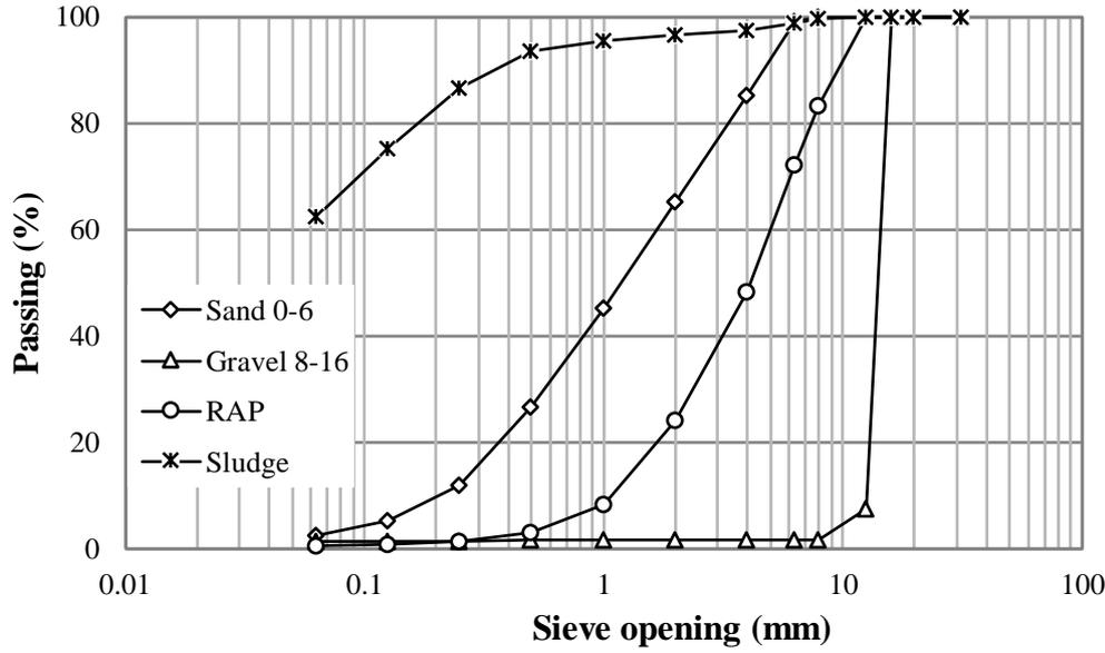
Fig. 1. Particle size distribution of aggregates, RAP and mineral sludge
