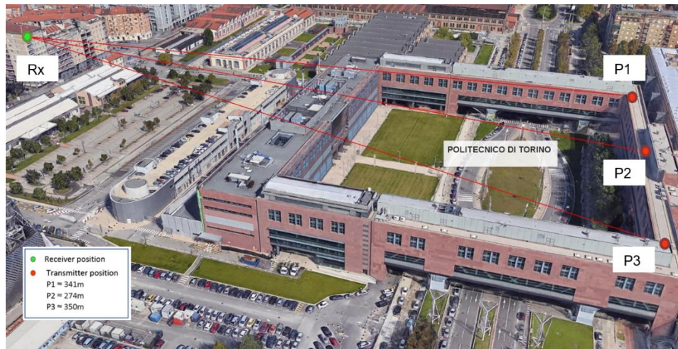
Figure 1. Setup 1. Position of the transmitters (P1, P2, P3) and of the receiver (Rx) with relative distance.
