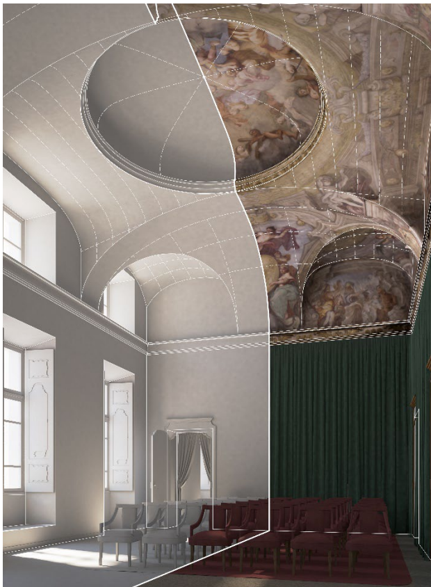
Figure 19. Superimposition of SfM 3d model and interpretative geometric model of 'Camera grande del letto' (Modelling: F. Natta)
