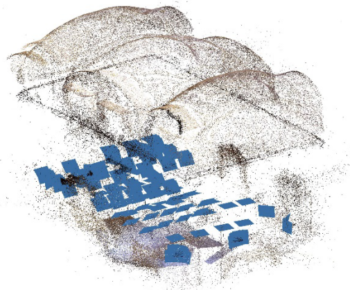
Figure 7. Sparse point cloud with aligned cameras from PhotoScan - 'Prima Anticamera' (Modelling: F. Natta)
