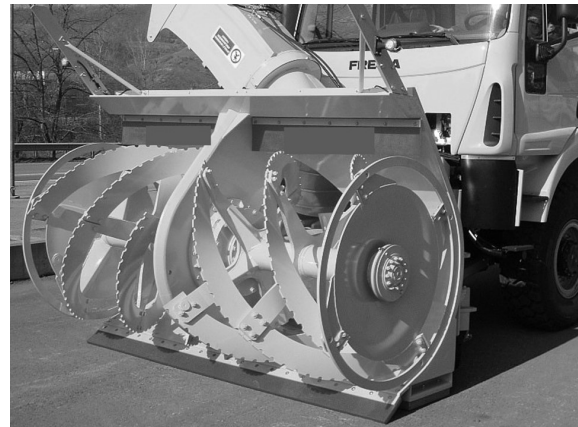
Figure 2. Snowplow mill considered as case study
