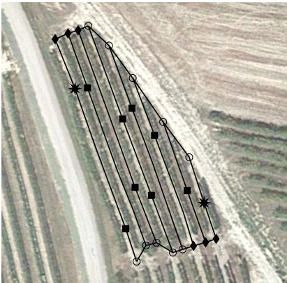
Fig. 1. An example of undirected graph that represents the POIs and the available paths for the UGV on a real vineyard for the case N = 16 nodes.
