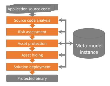
Figure 2.1: ESP workflow.
