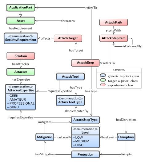
Figure 3.4: UML class diagram of the attack meta-model.
