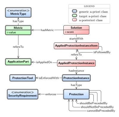
Figure 3.3: UML class diagram of the protection meta-model.
