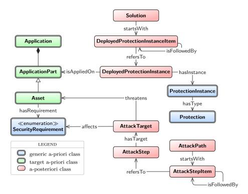
Figure 3.1: UML class diagram of the core meta-model.
