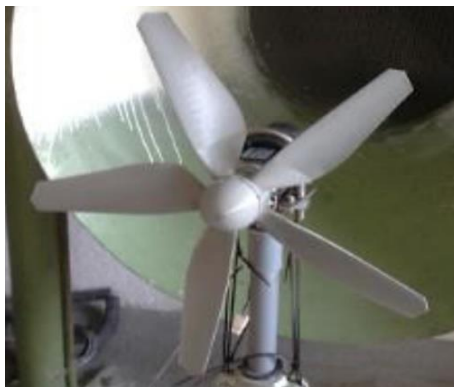
Fig. 1. The 3D model of the wind rotor under test
