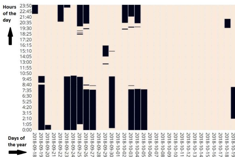
Fig. 6 Measured fan-coil actuator openings (0 closed, 1 open) between 18 September 2018 and 19 October 2018 in one of the four monitored guest rooms at Hotel Residence L’Orologio. The colour scale has only 2 colours: beige for periods with closed actuator and black for periods with open actuator
