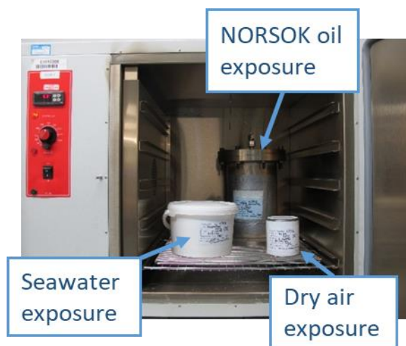
Figure 3-2: experimental setup for the accelerated exposures in electric oven.
