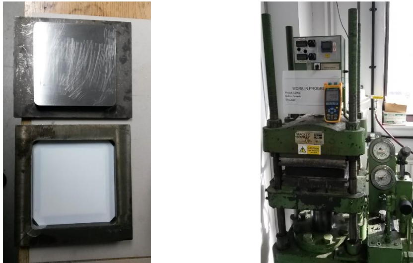
Figure 3-1: the open small mould (the PTFE cover sheets and rubber rim are visible), on the left, and the hydraulic press used for the compression moulding, right.
