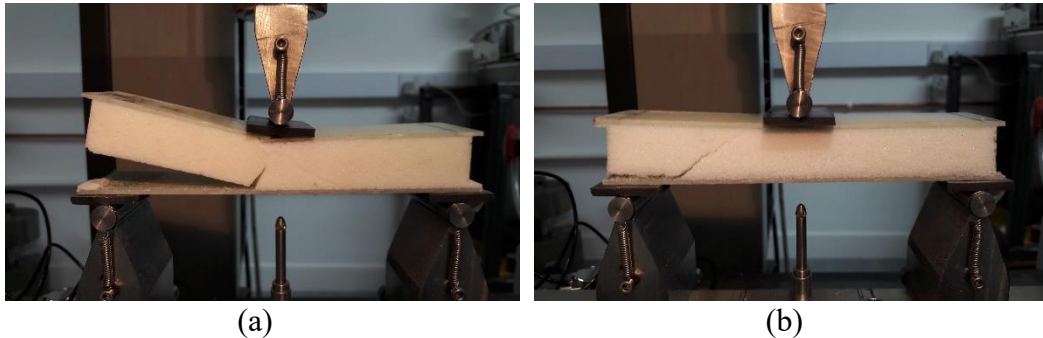
Figure 5-22: 3PB broken sandwich specimens after unloading. (a) from batch #12, (b) from batch #14.
