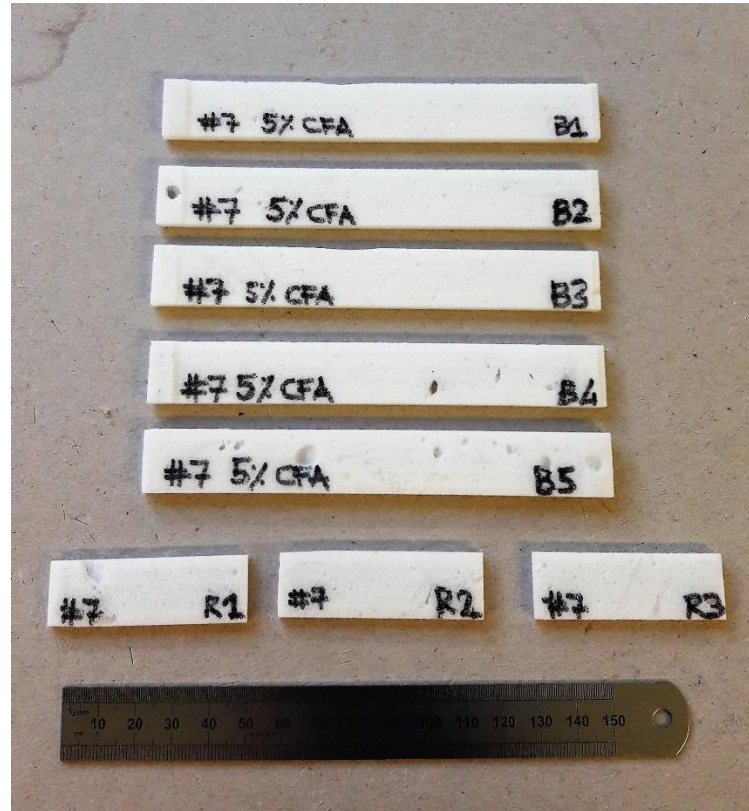
Figure 5-10: the epoxy foam specimens for the quasi-static three-point bending and DMA tests.
