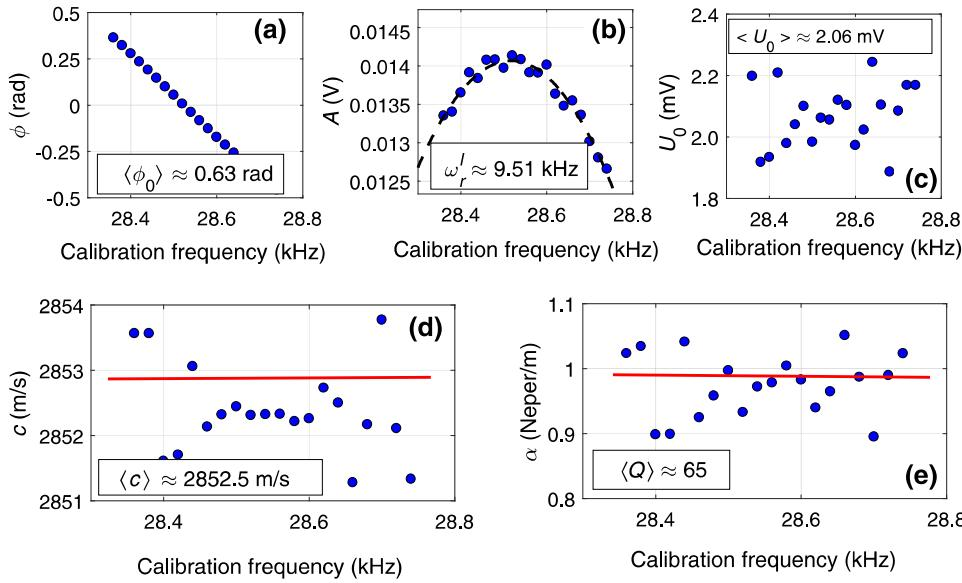
FIG. 3. Results of the calibration procedure performed. All quantities are reported as a function of the calibration frequency. (a) Phases ( $\phi = \Phi - \phi_0$ ); (b) amplitudes ( $A$ ); (c) calibration amplitude ( $U_0$ ); (d) estimated velocity; (e) estimated damping. Red lines in the last two subplots represent the values measured in independent experiments using TOF observations and reverberation decay.
