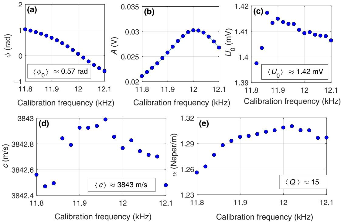
FIG. 5. Results of the calibration procedure performed for the concrete sample B06. All quantities are reported as a function of the calibration frequency. (a) Phases ( $\phi = \Phi - \phi_0$ ); (b) amplitudes ( $A$ ); (c) calibration amplitude ( $U_0$ ); (d) estimated velocity; (e) estimated damping. Distance correlation coefficients [39] are 0.6, 0.45, and 0.62 for  $U_0$ ,  $c$ , and  $\alpha$ , respectively.
