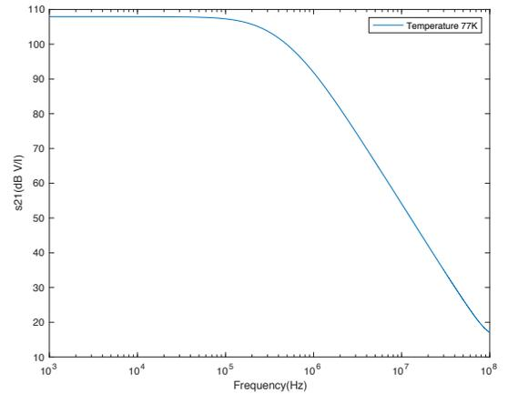
Fig. 7: AC response of the Folded Cascode single-ended.
