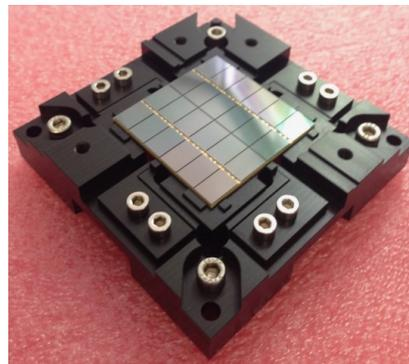
Fig. 1: A 24 cm<sup>2</sup> SiPM tile developed by the Darkside Collaboration.
