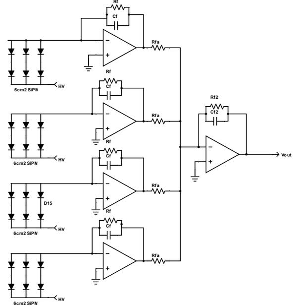
Fig. 3: Simplified schematics for the readout of 4 quadrants
