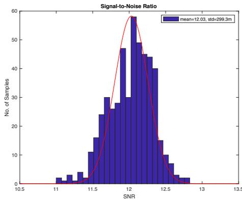
Fig. 8: Montecarlo simulation of Folded Cascode, signal-to-noise ratio.
