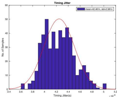
Fig. 9: Montecarlo simulation of Folded Cascode, timing Jitter.
