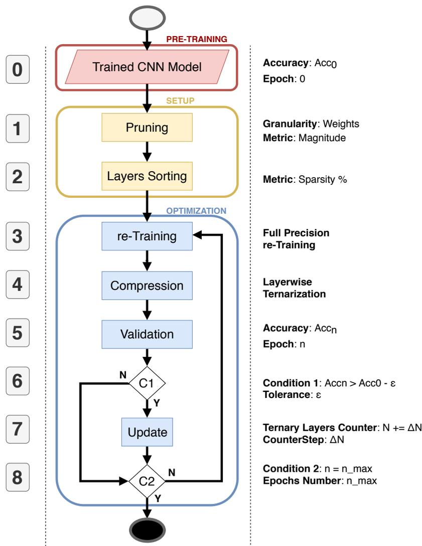
Figure 4. The proposed net compression pipeline.
