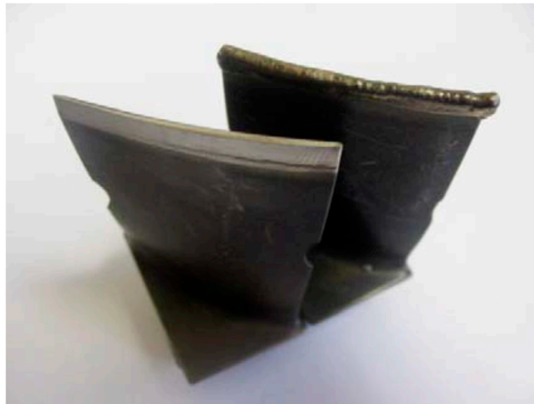
Figure 16. Thin-curved compressor blade before and after repairing [91].
