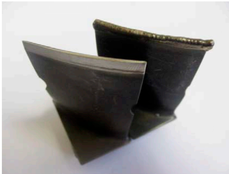
Figure 16. Thin-curved compressor blade before and after repairing [91].
