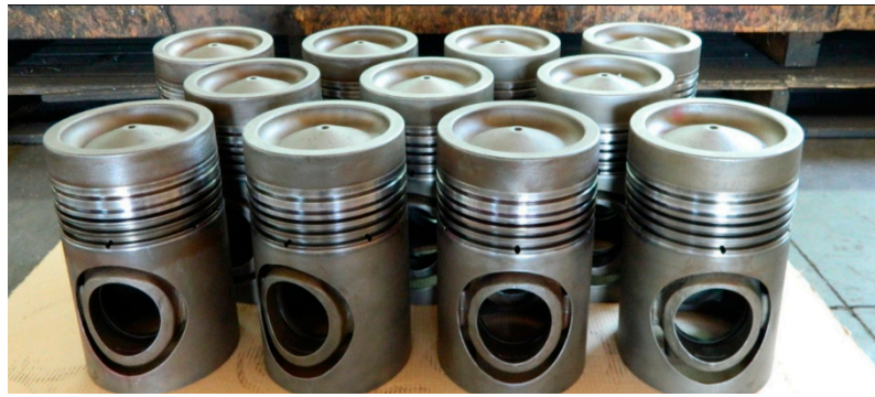
Figure 12. Four-stroke pistons repaired by DED (Courtesy of KIMI) [88].
