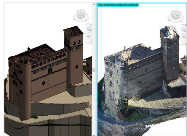
Figure 6. Point cloud usage for supporting modeling stage
