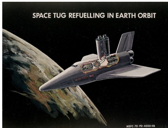
Figure 2.12: The rendering of a space tug refueling operation through one Shuttle orbiter (credit: NASA).
