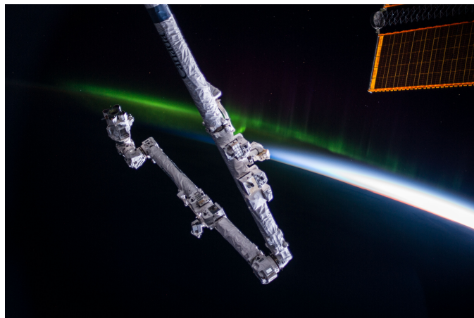
Figure 2.7: Canadarm2 attached to the ISS with an aurora in the background. (credit: NASA).
