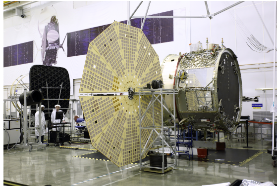
Figure 2.18: The Cygnus spacecraft with its cymbal-like UltraFlex solar arrays deployed (credit: NASA).
