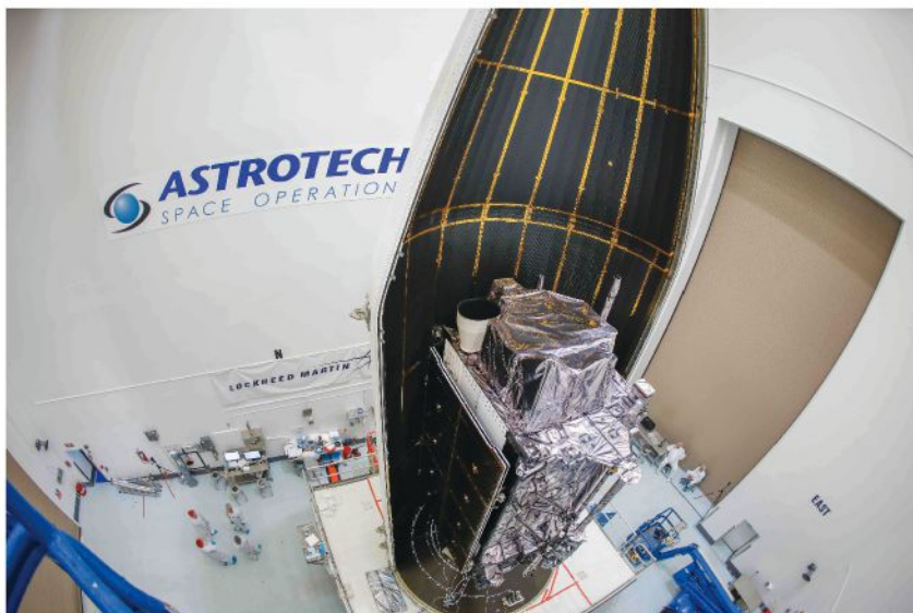
THE SECOND GPS III satellite is encapsulated in preparation for launch on August 23.
