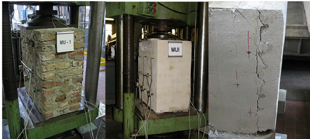
Figure 7: Compression test of: (a) original masonry specimens (MU); (b) masonry specimens strengthened by injection technique (MUI); (c) masonry specimens strengthened by jacking wall technique (RMA).
