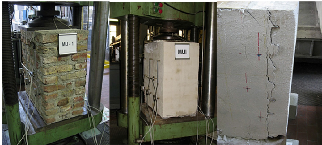
Figure 7: Compression test of: (a) original masonry specimens (MU); (b) masonry specimens strengthened by injection technique (MUI); (c) masonry specimens strengthened by jacketing wall technique (RMA).
