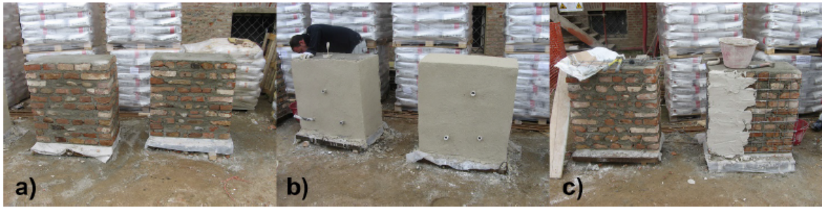
Figure 6: (a) Original masonry specimens; (b) masonry specimens strengthened by injection technique; (c) masonry specimens strengthened by jacking wall technique.
