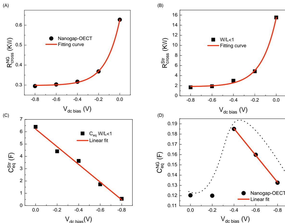
**Figure 5.** Resistive contribution to the total impedance at the crossover between a regime where the electrochemical response is controlled by charge transfer mechanisms and a regime showing a diffusion limited behavior in the case of (A) a Nanogap-OECT and (B) a stripe-like OECT.  $C_{eq}$  as a function of  $V_{dc}$  bias for (C) a stripe-like OECT and (D) a Nanogap-OECT. The related fitting curves (red curves and lines) are reported in all cases.
