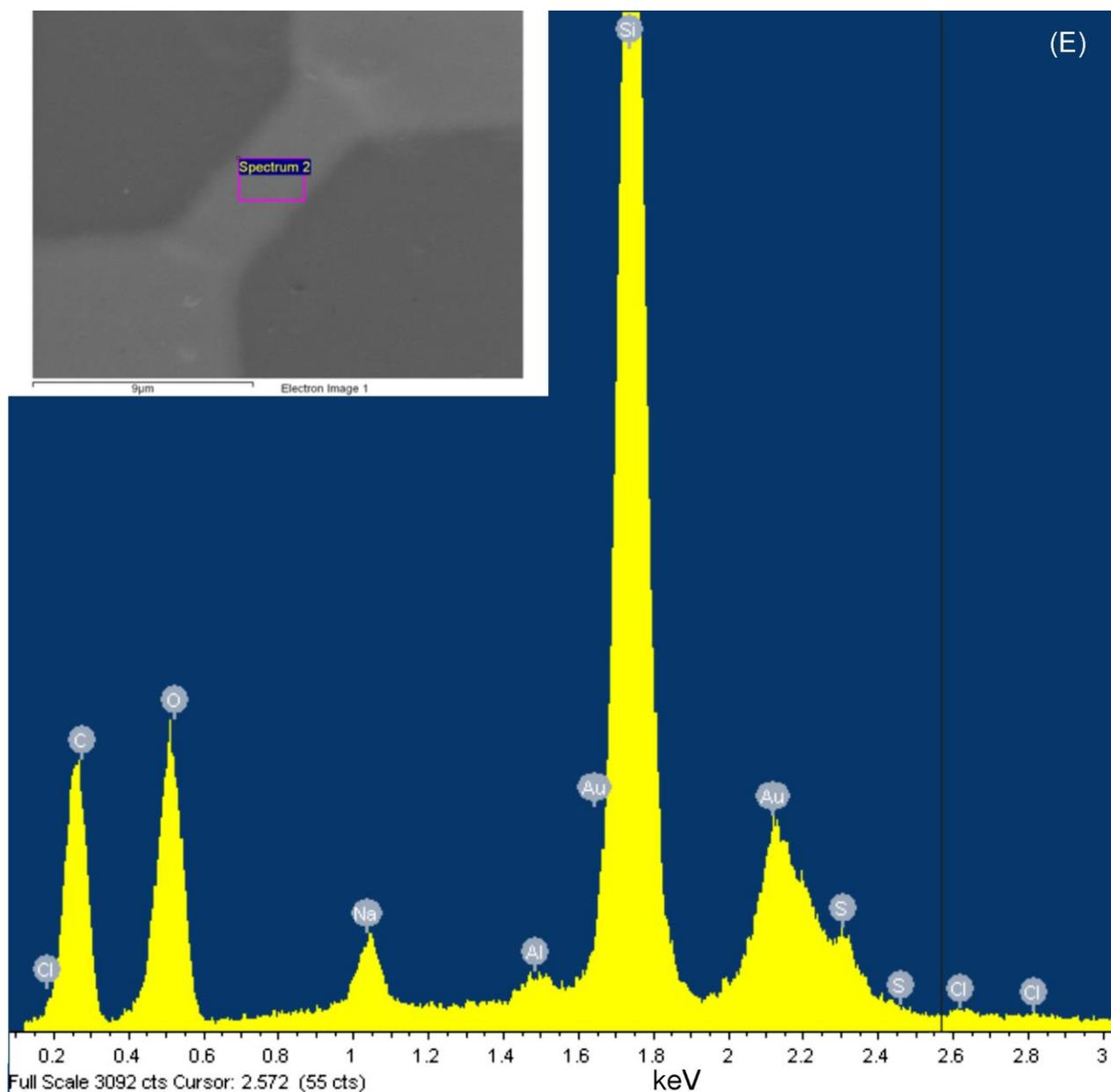
**Figure 1.** (A) Au microwire (8 μm in length and 2 μm in width) fabrication by Au/Al<sub>2</sub>O<sub>3</sub> deposition and patterning; (B) Nanogap formation by EIBJ; (C) contacts passivation; (D) PEDOT:PSS deposition and patterning; (E) EDS spectrum of the central area of the final Nanogap-OECT characterized in NaCl electrolyte solution (in the inset the FESEM image of the investigation area).
