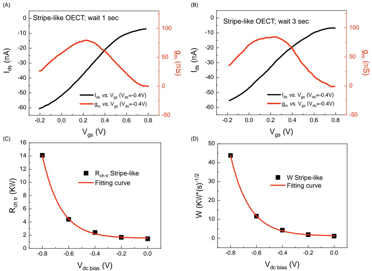
**Figure 7.** Transfer curves (black line) and transconductance (red line) as a function of  $V_{gs}$  for a stripe-like OEET at  $t_{scan} = 1$  s (A) and 3 s (B); (C) charge transfer resistance ( $R_{ch-tr}$ ) and (D) Warburg coefficient ( $W$ ) reported in Table 2 as a function of  $V_{dc}$  bias (fitting curves in red) for a stripe-like OEET.
