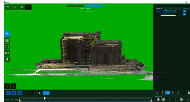
Figure 5. Misalignments between point cloud frames are visible after the acquisition, in yellow a single point cloud frame is highlighted
