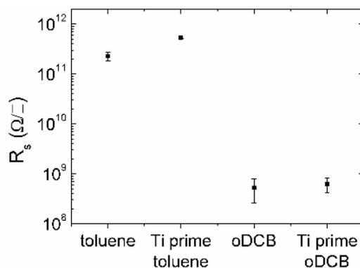
**Figure 3.** Sheet resistances measured on a set of minimum three devices for each kind of sample. Devices obtained from oDCB solution generally show a three-orders-of-magnitude improvement in conductivity, while samples treated with Ti prime show higher reproducibility for both solvents.
