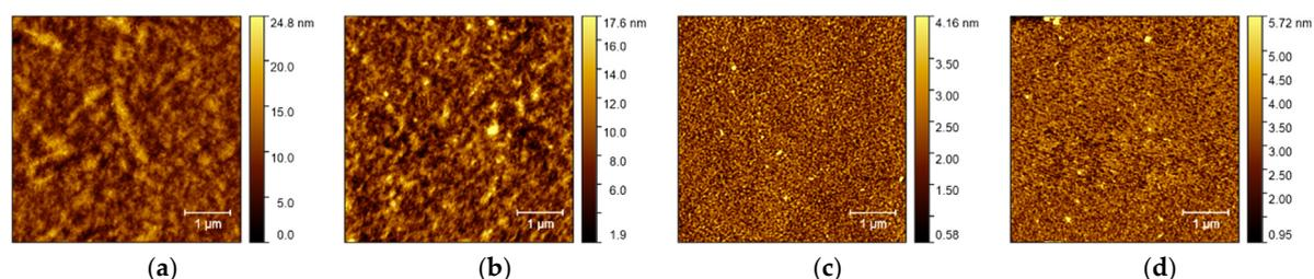
**Figure 1.** AFM images acquired in tapping mode of P3HT deposited on Si/SiO<sub>2</sub> substrate: (a) from toluene solution without adhesion promoter; (b) from toluene solution with Ti prime; (c) from oDCB solution without adhesion promoter; (d) from oDCB solution with Ti prime.
