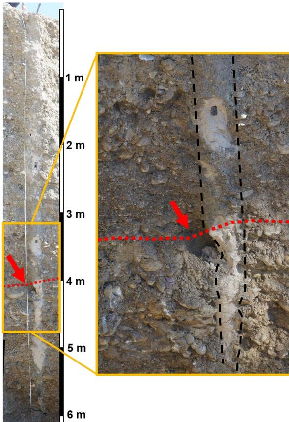
**Figure 12: Stratigraphic detail of the cemented geothermal probe. The red dashed line marks the interface between sandy gravels and the more compact conglomeratic layer with coarser grain size. The red arrows and the dashed black lines highlight the presence of empty spaces and discontinuities in the cementation below -4.10 m from the surface.**
