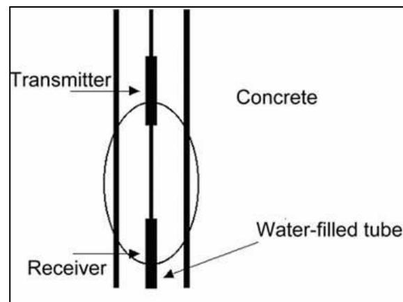
**Figure. 3 – Zoom on the instruments disposition during acquisition.**
