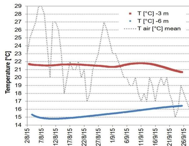
**Figure 13. Temperature monitoring inside the geothermal cemented probe at, respectively, -3 m (in red) and -6 m (in blue) from the surface. The daily mean air temperature is reported with the black dashed line.**
