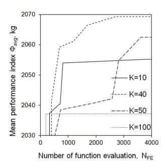
FIG. 7. Tuning of perturbation constant K (with B=1).
