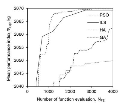
FIG. 14. Mean performance index  $\Phi_{avg}$  vs. number of function evaluation  $N_{FE}$ .
