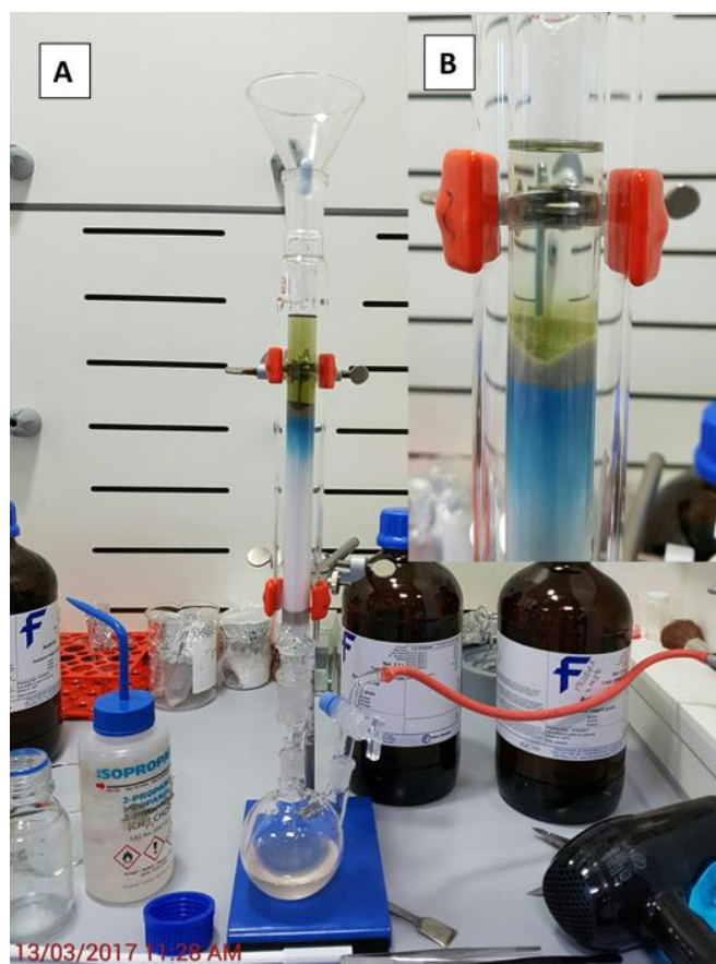
Figure 4.6: a) Separation column for removing copper from the polymer solution, b) an up-close look at the color change as \text{CuCl}_2 forms a complex with \text{Al}_2\text{O}_3
