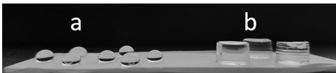
Figure 2.14: Hydrogel samples fabricated for characterization, a) 30 \mu\text{L} beads with 4 mm diameter, b) 200 \mu\text{L} beads with 7.5 mm diameter and 5 mm height.
