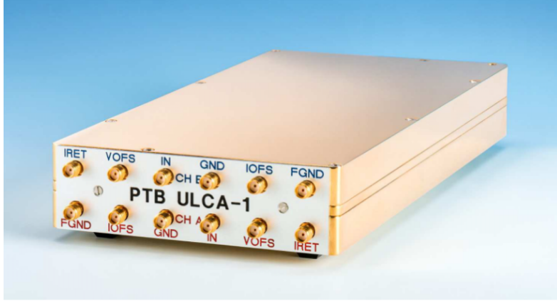
Figure 3.5: A two-channel standard ULCA. Reproduced from [18], with the permission of AIP Publishing.
