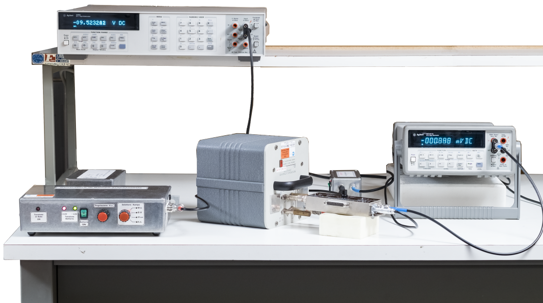
Figure 4.3: Picture of the calibration set-up corresponding to the schematic of figure 4.2. Bottom left: source G with its power supply. Centre: C , A and trigger. Top left: V_{\text{in}} . Right: V_{\text{out}} . Note that the amplifier A and the capacitor C are directly connected to reduce possible effects of dielectric absorption in the insulating materials of the connection. Reprinted by permission from [141] © 2018 IEEE.
