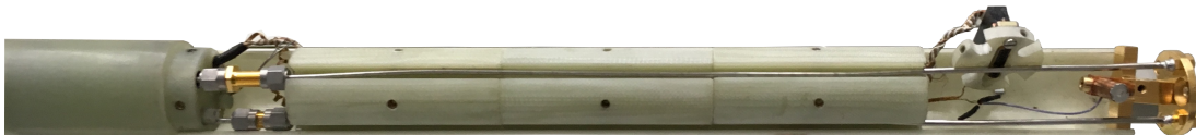
Figure B.5: Picture of the line A (top) and line B (bottom) in the Section II. In the picture are clearly visible the SMA (left) and SMP (right) connectors and two adaptors.
