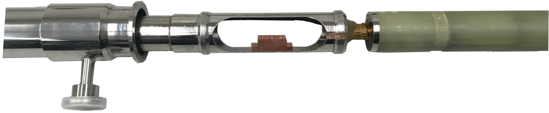
(a) Picture of the 1K-pot region. It is also shown the cavity used to thermalize the cables with the first prototype of thermalization box (section B.4.4).
