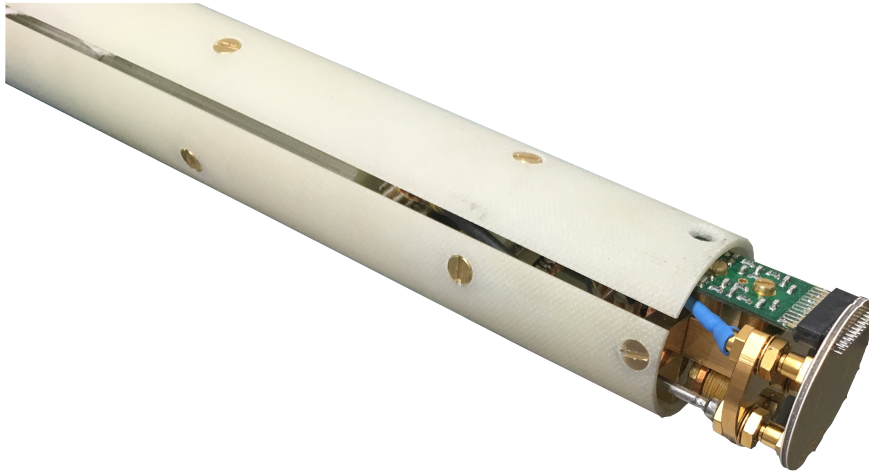
Figure B.8: Picture of the terminal part of the probe. It shows the RF lines (bottom), the signal lines (top), the low-pass filter PCB and the sample holder.
