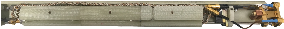
Figure B.7: Picture of the signal lines and the 24 DC lines. For what concerns the signal lines are visible the wrapped Thermocoax® and the Lemo cables reaching the sample holder. For the 24 DC lines the woven loom wires and the connector are shown.
