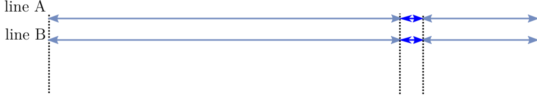
Figure B.4: Scheme of the RF line assembly: in light blue is represented the position of the stainless steel cables while in blue the location of the NiTi cables.
