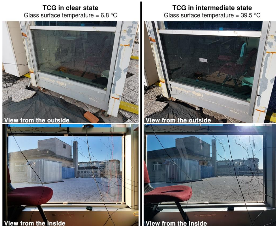
Figure 6. Views from outside (upper band) and inside (lower band) of a thermochromic glazing with the same characteristics as the sample analysed. The pictures are relative to the component in its clear state (left) and in an intermediate state, relative to a glass surface temperature equal to 39.2 °C (right).
