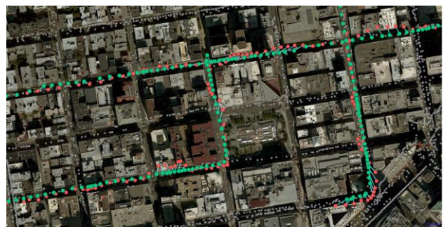
Figure 1. Original photo locations (in red) and corrected locations (in green) estimated through a photogrammetric approach
