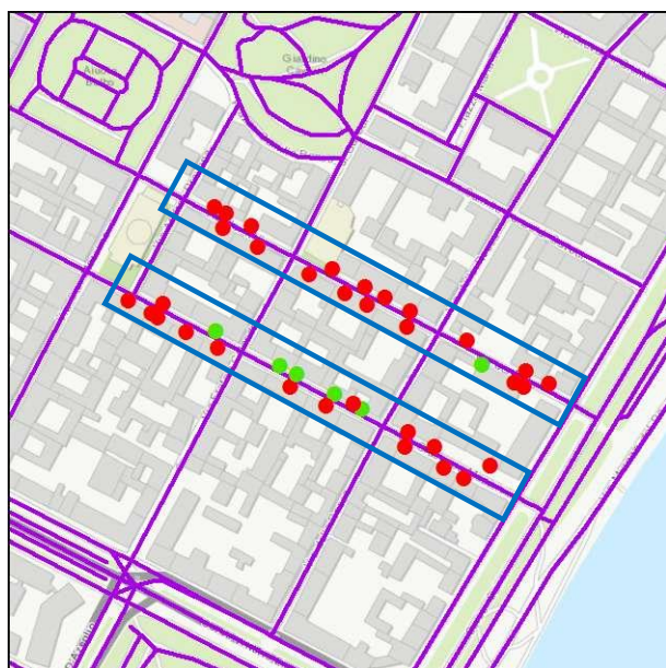
Figure 14. “PASSO CARRABILE” traffic signs in the test area (blue rectangle): actual positions (red dots) vs Mapillary detections (green dots)
