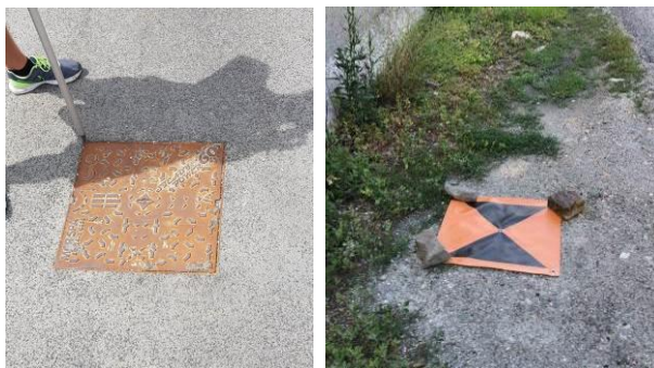
Figure 6. Examples of existing (left) and artificial (right) markers measured on the ground and used as GCP and/or CP.
