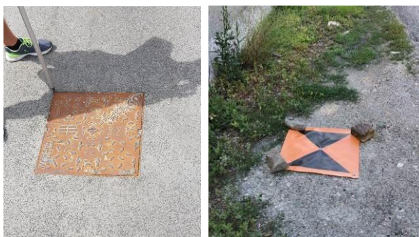
Figure 6. Examples of existing (left) and artificial (right) markers measured on the ground and used as GCP and/or CP.
