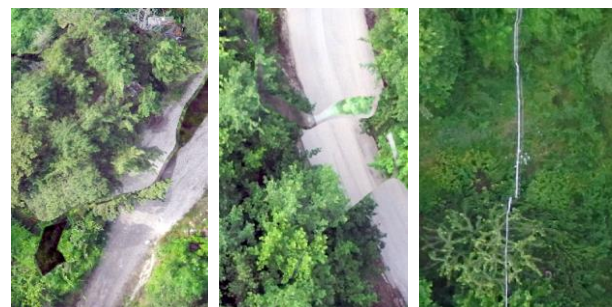
Figure 11. Example of mosaicking issues in areas with dense/high vegetation
