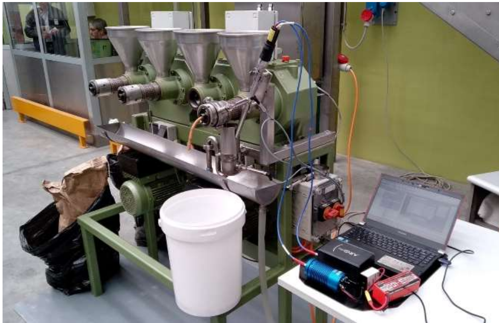
Figure 5-19. Expeller press equipped with a thermocouple and an in-house assembled portable FT-NIR instrument equipped with a fibre optic transfectance probe.
