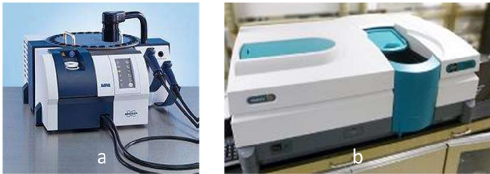
Figure 5-20. FT-NIR MPA spectrometer from Bruker optics (a) and Varian Cary 5000 UV-Vis Spectrophotometer (b).
