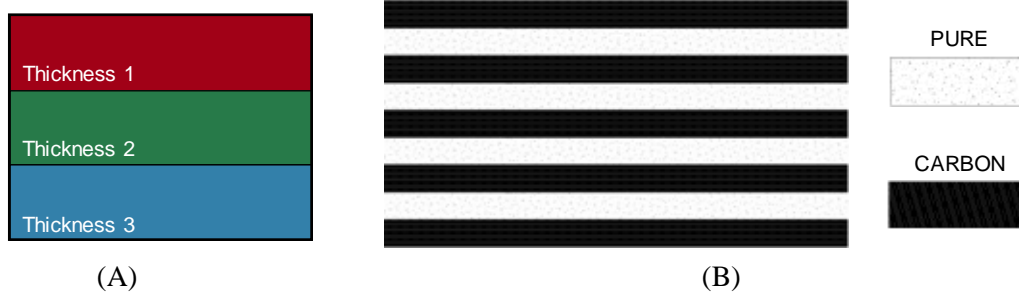
Figure 1: On the left-hand side (A) top view of the sheet used for the production of the specimens, on the right-hand side (B) example of the stacking sequence of the hybrid lamina used for the tensile and three-points bending specimens
