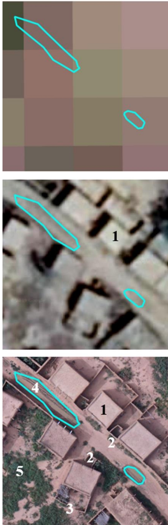
Figure 3. Touré, 2018. Images for exposed items' identification: Sentinel satellite image with 10 m resolution (top); satellite high-resolution image freely available from Google Earth showing (1) earth construction (center); very high resolution image taken from a UAV showing (1) hearth house, (2) latrines, (3) house entrance, (4) ephemeral water body, (5) millet (bottom).
