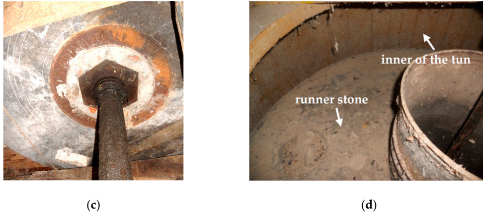
Figure 17. Coupling between the shaft C and runner stone: (a) Shaft C (Riviera mill); (b) runner stone (Riviera mill); (c) shaft C (Forno mill); (d) runner stone (Forno mill).
