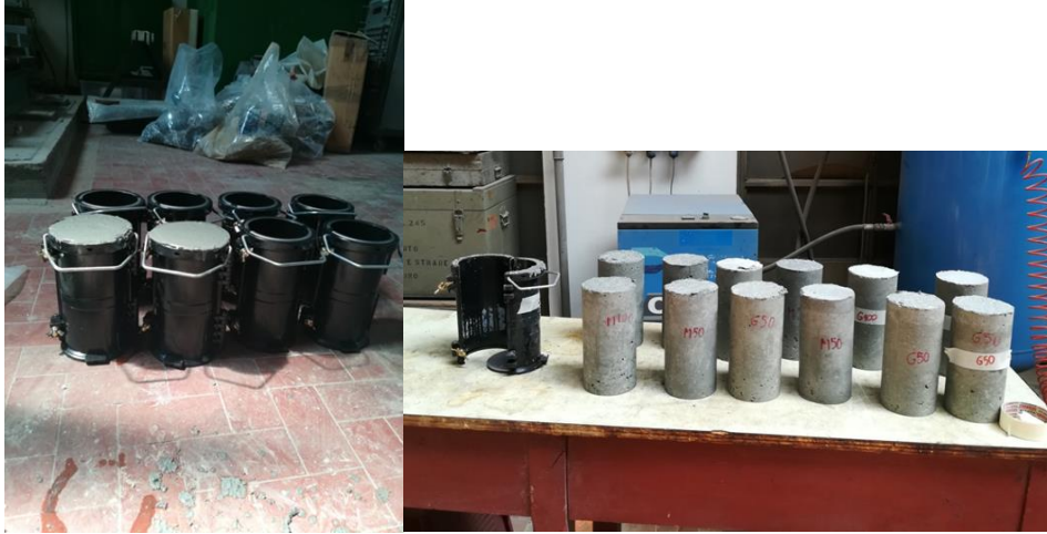
Figure 103: Left: cylindrical specimens holder with dimension 200mm height and 100mm diameter. Right: specimens obtained after 24 hours of curing.
