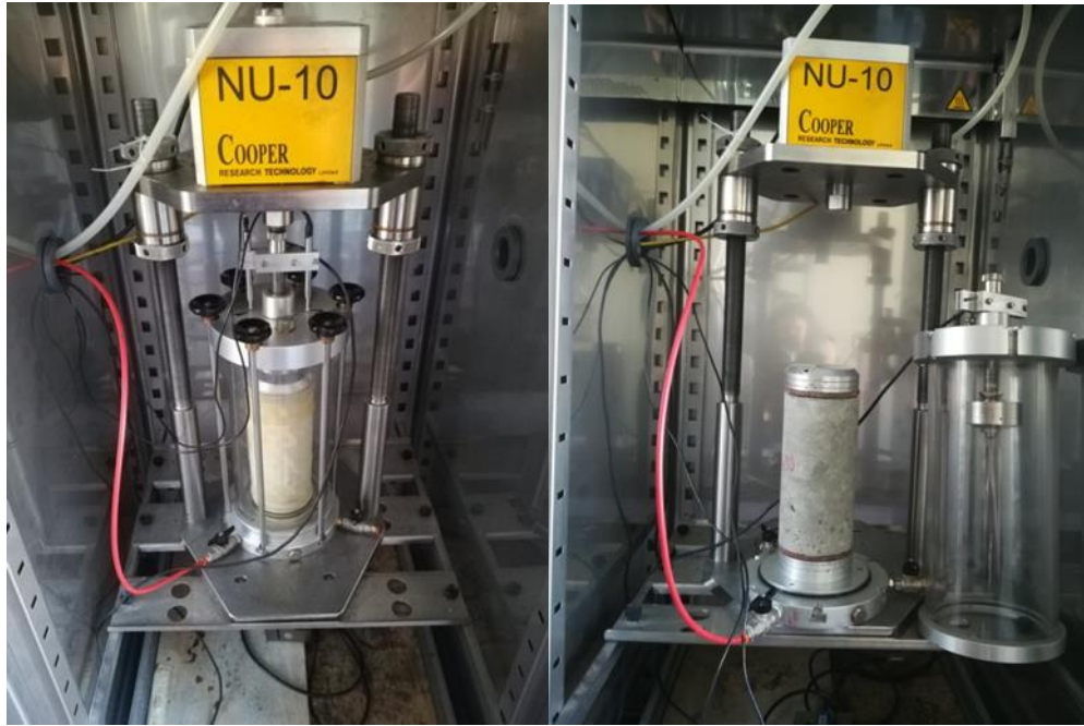
Figure 106: Specimen in the triaxial cell device.
