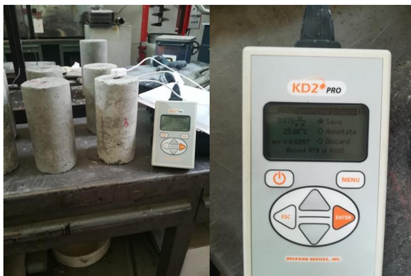
Figure 116: Device KD2 PRO used for thermal conductivity measurements.
