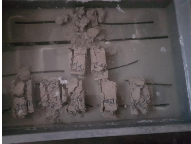
Figure 136: Water absorption of L1, L2, T1 and T2 specimens after salt crystallization cycle and flexural strength test. Specimens breakdown.
