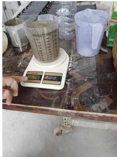
Figure 129: Bulk density of fresh mortar.
