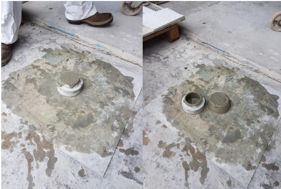
Figure 130: Spreading test on fresh mortar, with Hargerman cone.
