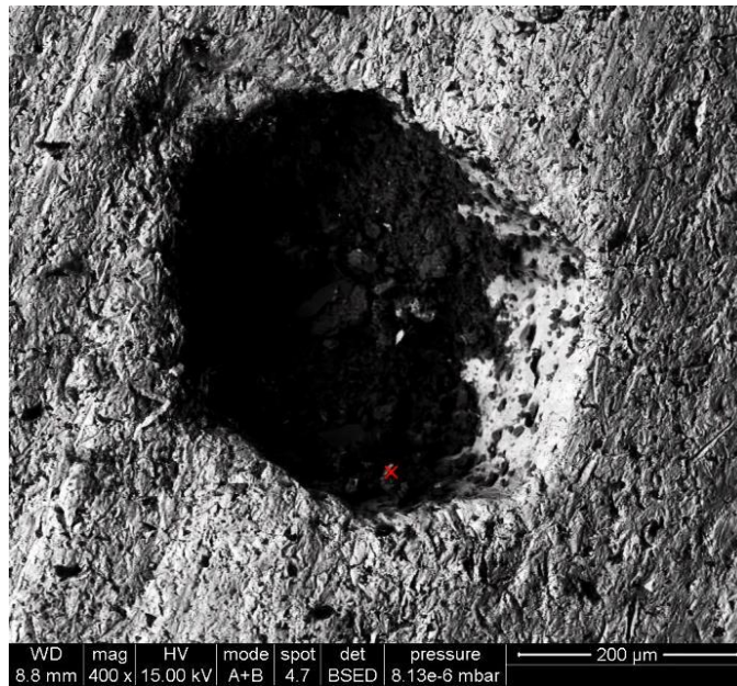
Figure 70: SEM EDS analysis of diamond blade segment matrix used in plant MCD. Magnification 400X. Scaled diamond.
