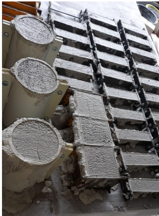
Figure 128: Plaster specimens prepared for physical- mechanical tests, according to standard UNI EN 998-1 and 2.
