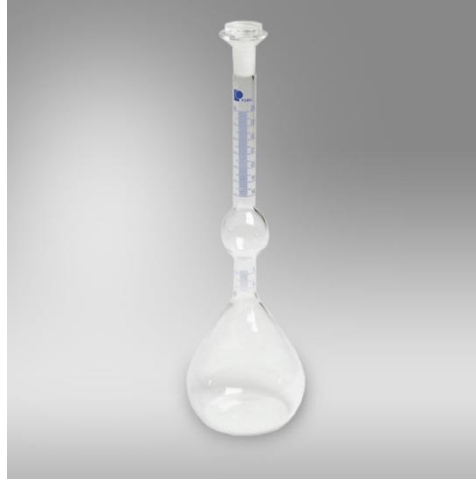
Figure 95: Le Chatelier Flask according with standard EN 196-6 Methods of testing cement. Determination of fineness. (Source: http://multiserv-morek.pl/en/products,cement,le_chatelier_flask_en_196-6 )
