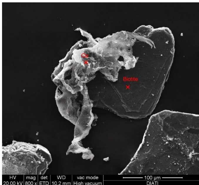
Figure 77: SEM photo of MVG magnetic fraction sample. Biotite covered by cobalt metal part.
