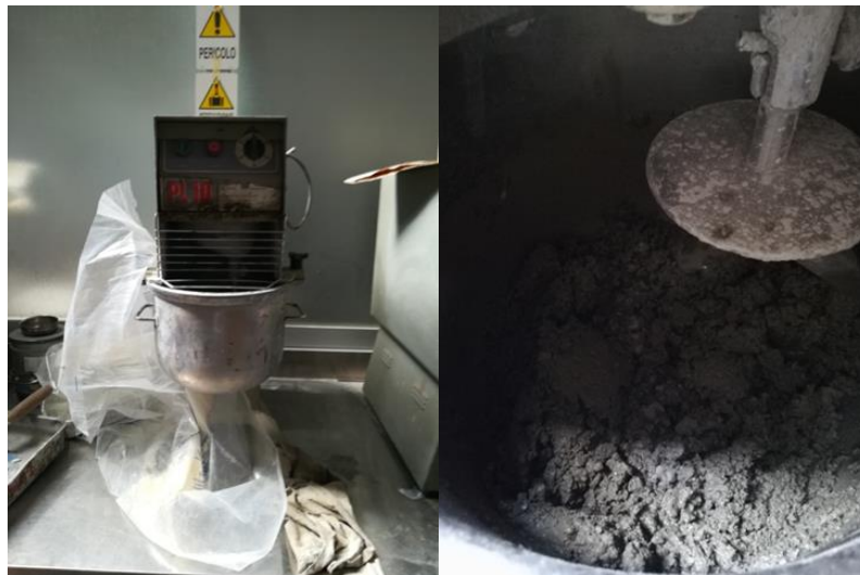
Figure 102: Left: mixing device used. Right: homogenous mix obtained.
