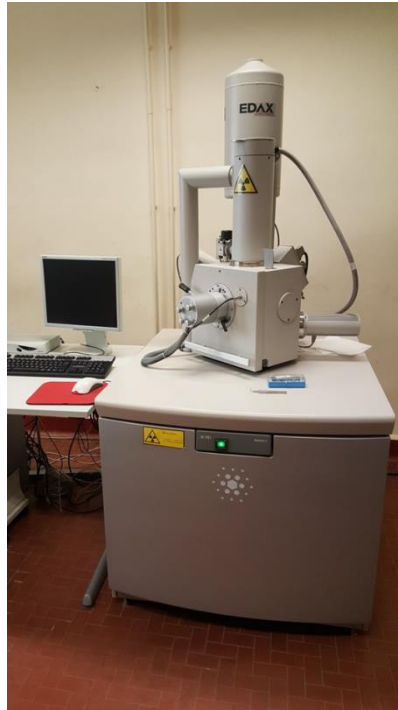
Figure 60: SEM FEI model Quanta Inspect 200 LV with energy dispersive X-ray spectroscopy (EDS) using EDAX Genesis with the SUTW detector, in use in Laboratory of DIATI Department in Polytechnic of Turin.
