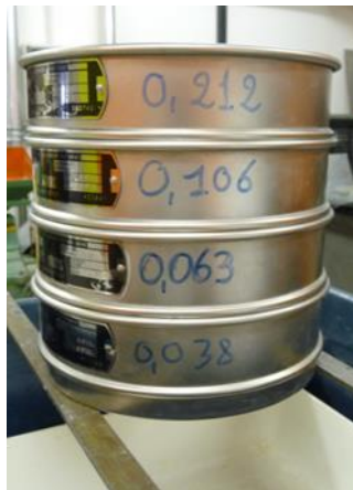
Figure 42: sieves column used for the particle size distribution of sludge.
