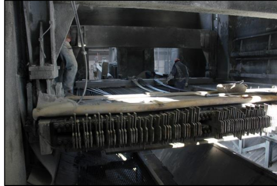
Figure 12: Gangsaw machine for hard cutting stones.
