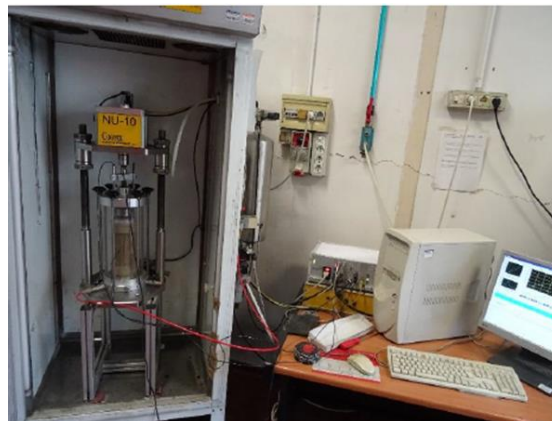
Figure 105: Triaxial cell with repeated load device used for the test.
