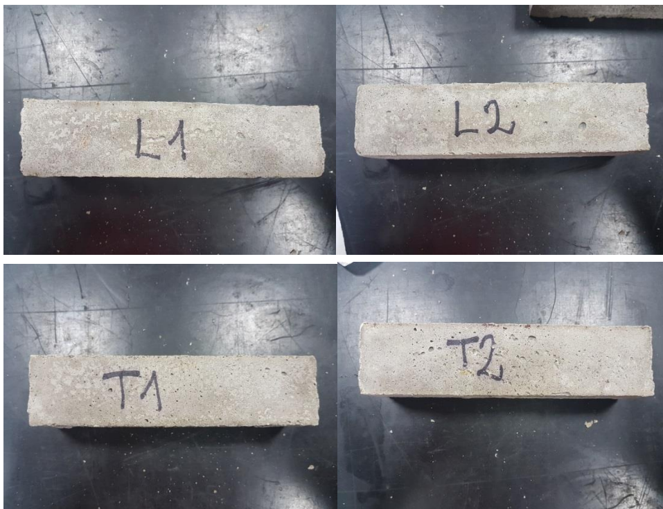
Figure 135: Specimens after salt crystalization cycle.
