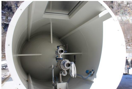
Figure 25: Internal view of a tank for a filter press system
