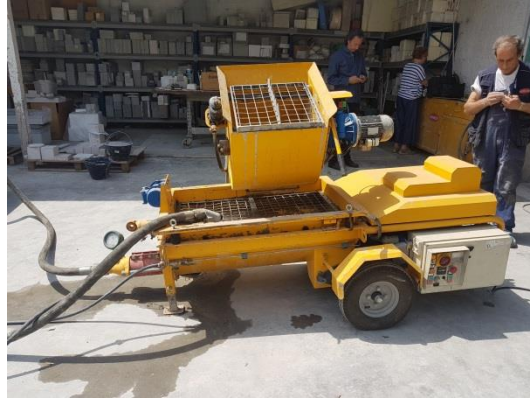
Figure 125: S8 EVM machinery creation of TEK.SP.ED s.r.l. used for eco-mortar for plaster mix design.
