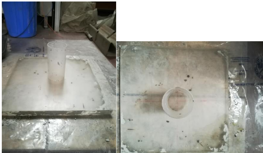
Figure 99: Standard cylindrical mold for the execution of the flowability test
