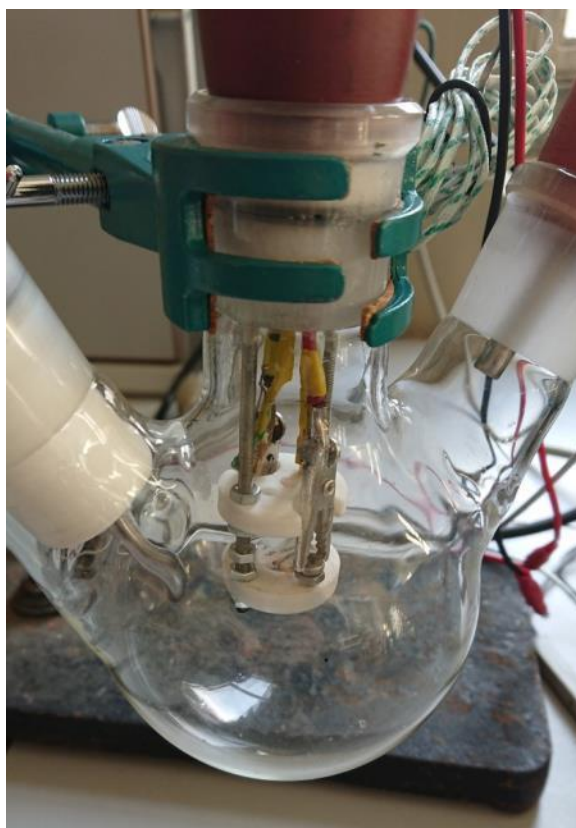
Figure 6. Three-neck flask where sensor and sample are arranged
