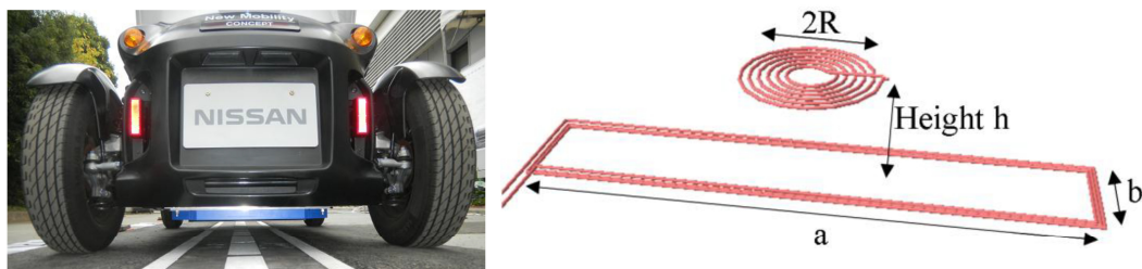
Fig. 1.14: Nissan dynamic WPT prototype; on the left: Photograph of the test EV, and on the right: structure of the coils.
