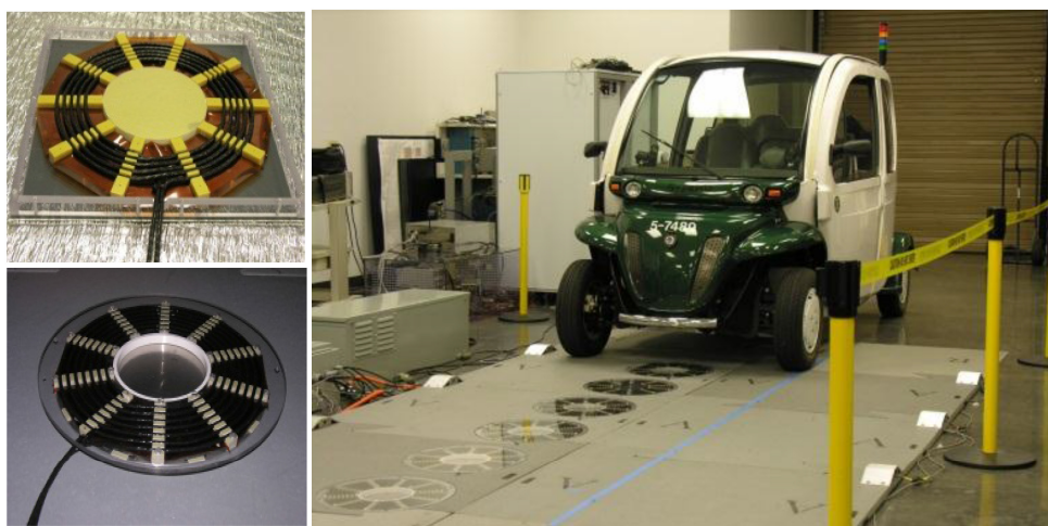
Fig. 1.17: The ORNL dynamic WPT charging of an EV.
