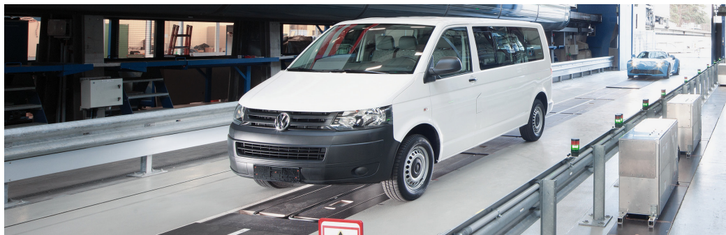
Fig. 1.15: INTIS dynamic charging setup.
