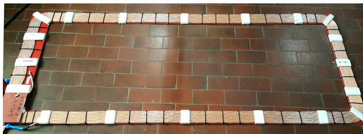
Fig. 5.6: Picture of the transmitter coil with 10 turns.
