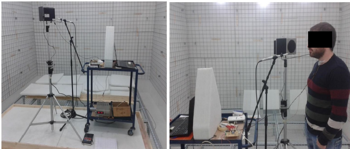
Fig. 1.2 Measurement setup: air and contact microphone, acoustic source, conditioning circuits, acquisition board and PC.
