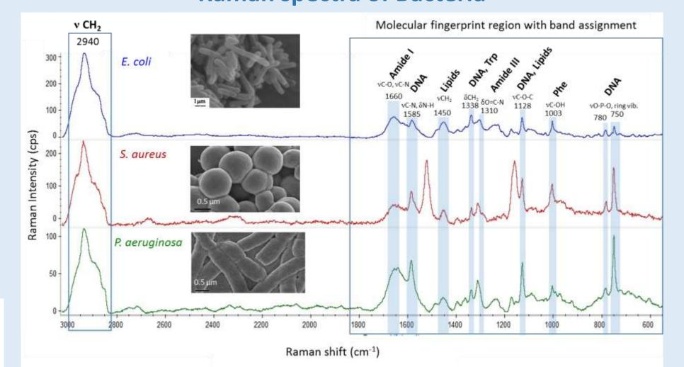
Raman characterization of: E.coli, S. Aureus and P. Aeruginosa using our DEP device. Optimized setup conditions for the cell: sinusoidal wave V = 5 Vpp, f = 800 kHz, aggregation time: 360 s. Optimized setup conditions for Raman microscope: laser line: 532 nm, laser power: 10 mW, objective: 60x water immersion, integration time: 2.5 s for 24 scans (1 min per spectrum).
