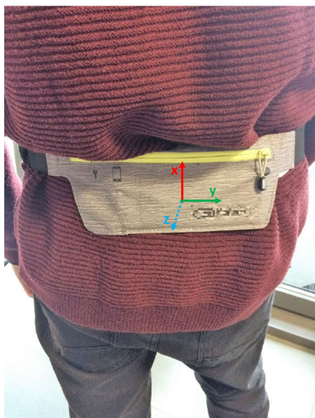
Fig. 7 Experimental setup for FOG detection
