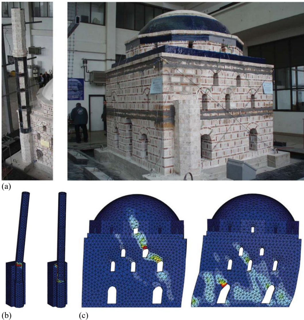
Figure 26: Models of the Mustafa Pasha Mosque in Skopje, (Portioli et al., 2011): (a) physical model with strengthening; (b) distribution of plastic strains at the collapse in the minaret before, (left), and after, (right) the strengthening; and (c) distribution of plastic strains at the collapse in the mosque before, (left), and after, (right) the strengthening.
