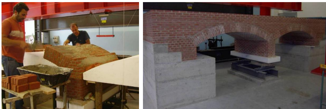
(a) (b) Figure 12: Physical model of masonry arch bridge, (Ruocci, 2010): (a) model during the construction; and (b) final model.
